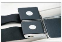
ABOVE LEFT: Seat belts — the female ends — were stored on clips attached to the center console; the male ends were stowed inside retractable units between the seats and the doors. Government standards required that all passenger cars be equipped with front seat belts starting in the 1965 model year.
