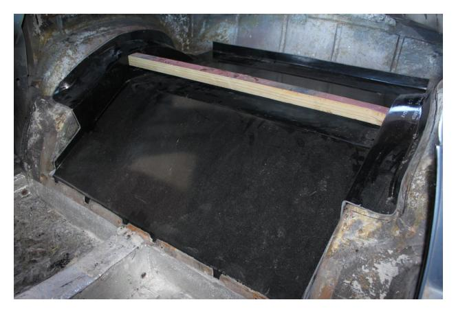
Wood support for Conv ONLY. Width of support used is 37 5/8" This may vary slightly because of factory tolerances.
