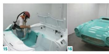
15 Once all of the unseen work was completed, it was finally time to apply the shiny stuff. The Cascade Green was matched to the color found underneath various interior panels and was mixed by Chris from Automotive Paint and Supply to ensure accuracy.
