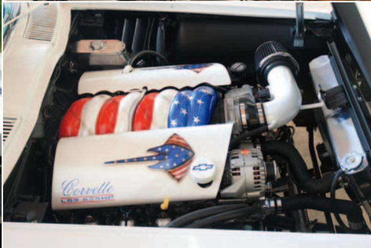
ABOVE Larry enjoys MUCH better fuel mileage from his 525-hp LS3 engine. TOP CENTER The chassis has been swapped for a Street Shop unit, giving much better handling, performance and braking than the original while requiring no modification to the underside of the body.
